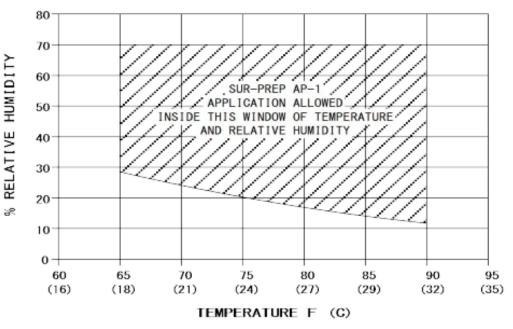
NOTE: THE TEMPERATURE AND HUMIDITY RANGES SHOWN ARE THE LIMITS FOR APPLICATION TO ASSURE OVERCOAT TOPCOAT ADHESION. THESE LIMITS DO NOT TAKE INTO ACCOUNT EQUIPMENT CONTROL TOLERANCES. DEPENDING ON EQUIPMENT SET POINT ACCURACY, IT MAY BE NECESSARY TO SET CONTROL LIMITS INSIDE THE LIMITS SHOWN IN THIS FIGURE.
